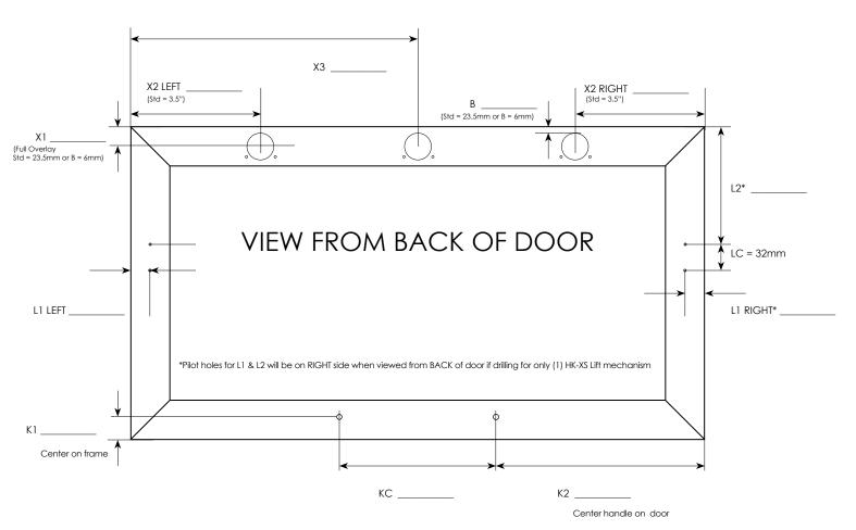
To locate L1 & L2 pilot holes for 20K4101 (wide frame) or 20K4101A (narrow frame) screw-on Door Mounting Plate:
