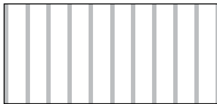
1/16" illuminated etched lines at 1/4" spacing
